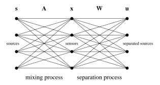
Figure 1: Blind source separation setup ( $M_s = M = 4$ ).
