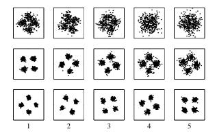
Figure 5: Constellation plot after convergence with  $M_{\rm s}=5$  4-QAM signals: (top) M=5, (middle) M=10, (bottom) M=20. The output signals  $u_m$  are sorted by their SNR.
