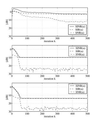
Figure 4: Convergence behavior of SNR ( $\mathbf{u}$ ), SIR ( $\mathbf{u}$ ), and SINR ( $\mathbf{u}$ ) for  $M_s=5$ : (top) M=5, (middle) M=10, (bottom) M=20.
