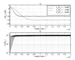
Figure 7: Performance of the blind separation algorithm A1 for  $M_s = 10$  sources. a) Performance measure  $J(\mathbf{P}_b)$  as described in section 4.1. b) Singular-value decomposition (SVD) of the permutation matrix  $\mathbf{P}_b$  for  $J_{\infty}(\mathbf{P}_b) = -20\,\mathrm{dB}$ .
