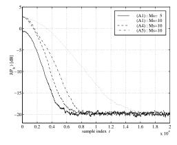
Figure 8: Performance of the combined blind/non-blind separation algorithms averaged over 30 runs. The step-sizes  $\mu$  are individually adjusted so as to result in the same separation degree  $J_{\infty}(\mathbf{P}_{\rm b}) = -20\,\mathrm{dB}$ : A1:  $\mu = 0.065$ ,  $\mu = 0.03$ , A4:  $\mu = 0.055$ ,  $\eta = 0.001$ , A5:  $\mu = 0.035$ .
